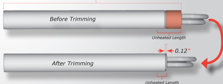
Heater size at Maximum Length Tolerance ( ALL cavity must be trimmed). 31.86"
